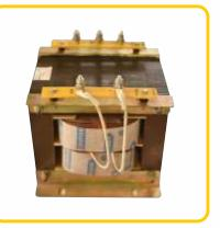
**5.** K Rated Transformers- A K-rated transformer is designed at a lower flux density as compared to a normal transformer, which is due to the fact that the third harmonic in the secondary winding causes a third harmonic current to circulate in the primary delta winding, increasing the flux density in the core. The core loss will be higher but it can be reduced by the use of additional core stack to the core.
