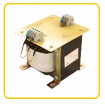
3. Control Transformers- A control transformer is an isolation transformer that provides good voltage regulation and is also designed to provide a high degree of secondary voltage stability (regulation) during a brief period of overload condition (also referred to as "inrush current"). Control transformers are also known as Machine Tool Transformers, Industrial Control Transformers or Control Power Transformers. We have the manufacturing capacity: up to 100KVA.
